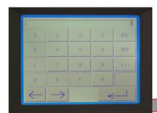
Access screen for selecting program memory and used for selecting numerical setting on machine
