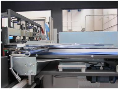
Belts are adjustable from both sides by loosening nut and turning hex bolt clockwise to <u>tighten</u> belt and counter clockwise to <u>loosen</u> belt.
