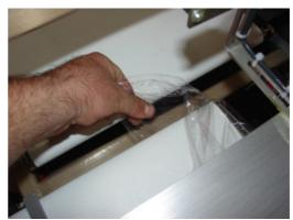
Using left hand move sheet from top side around the end of infeed conveyor going underneath conveyor and pull toward front of machine.
