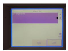
Low temperature on sealing bars will not allow the machine to operate
