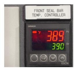
You may increase the temperature by pressing the up arrows key or decrease by pressing the down arrow key. The two buttons to the right are for programming functions only – Do Not Touch!
