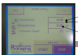
**-Front Portion-** Amount of film in front of package **-Photocell Delay-** Delays film feed after product is detected
