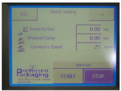
**Photocell Delay** – Photo eye will delay feeding of film in the event of 2 or more products are traveling down infeed together and they are not lined up even.
