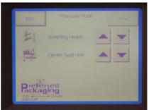
From main control panel use switch to raise or lower inverting triangle.
