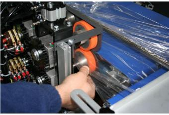
From the front of the machine grab both top and bottom sheets and feed into drive wheels
