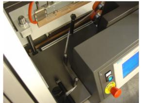
After having advanced the manual film feed several times take the excess film and feed through slot in scrap holder.
