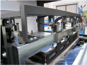
Safety sensor should be set 1/8" above metal bracket. Sensor gap should be set 3-4mm from bracket
