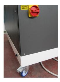
Machine has threaded casters that can be adjusted 10 from 90 to 100 cm maximum- working height is 900+ /- 50
