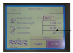
Seal Time- Amount of time cross seal stays down to seal film
