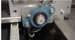
Grease in feed and discharge conveyor bearings utilizing the male fitting on the bearing
