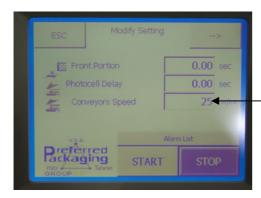
**Conveyor Speed-**From 0 to 25 meters per minute
