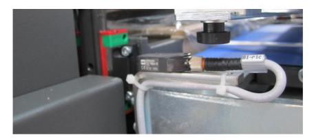
Top adjustment is for sensitivity minimum and maximum Bottom adjustment is for photo cell delay
