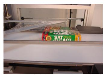
With product on infeed conveyor under inverting triangle adjust height.
