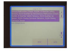
Sensor Malfunction: Safety sensors on seal head out of adjustment
