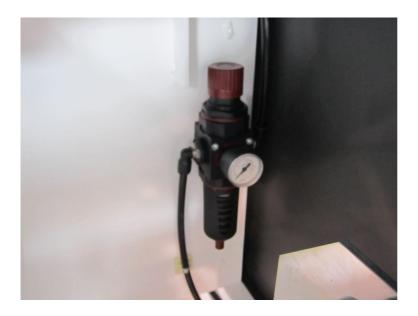
Connect air line to pressure regulator. Air gauge should be set at 6 bars = 80 PSI.
