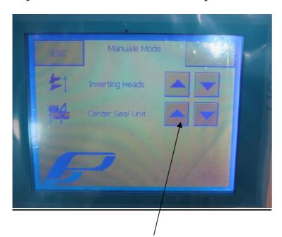
CENTER SEALING motorized adjustment from the touch screen
