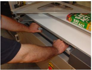
Using handles move conveyor in or outward until guide bar is near product.
