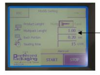
**Multi-pack Length** – Measure length of product in millimeters and add 5 mm to determine length of product. (1"-25.4mm)
